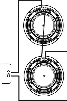
Four 4-ohm speakers @ 4-ohm series parallel
