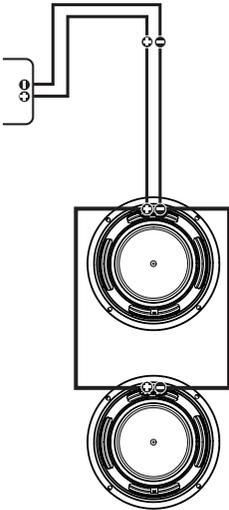
Examples of 4 ohm speakers in Series, Parallel and Series-Parallel wiring.
